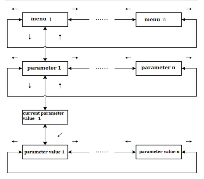
There are 4 directional keys 🗓 💆 to be used for the operation. 🗒 are used for horizontal movement in the same level menu and parameters. 🗒 are used for moving up and down through different level menus.
